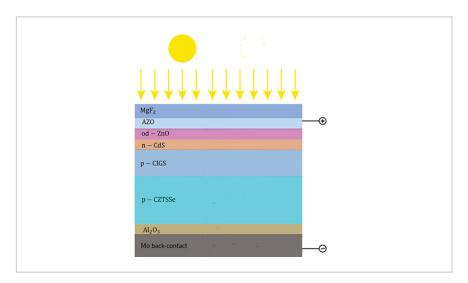
Double thin film layered solar cell
