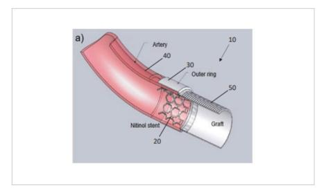
Figure 1: Configuration used in forming anastomotic devices
