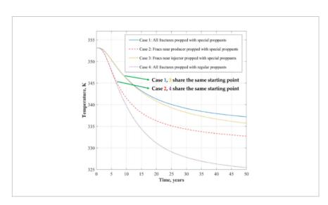
Temperature of produced fluid for different simulation cases using special proppants.
