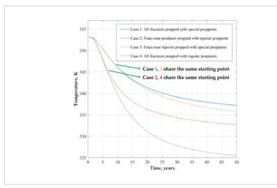
Temperature of produced fluid for different simulation cases using special proppants.
