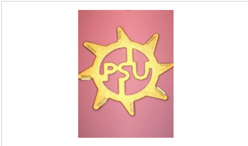
Microgear with Pt catalyst on teeth
