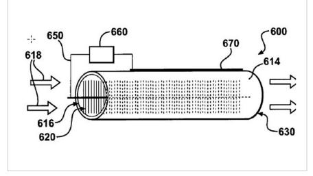
Tubular Cathode Encasing Electrode
