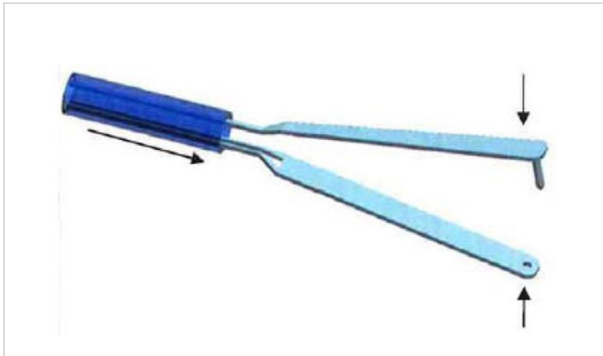
Sketch of endoscopic suturing device
