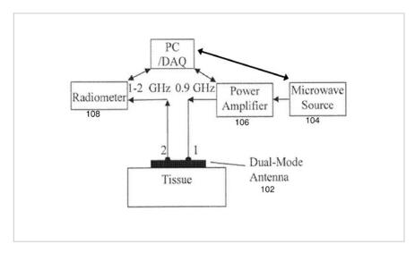
Diagram for microwave heating system
