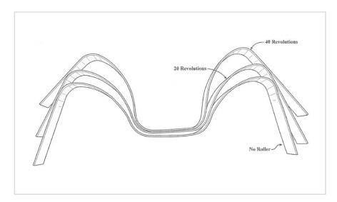
Roller Rotation Reduces Springback
