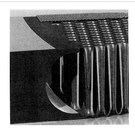
Example shell-and-tube heat exchanger
