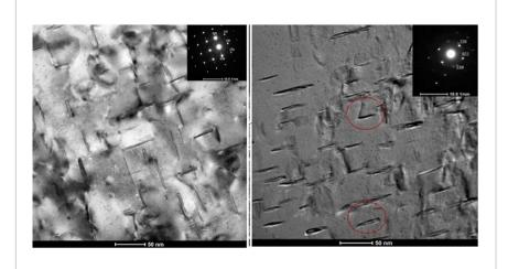
Electron micrographs of aluminum alloys
