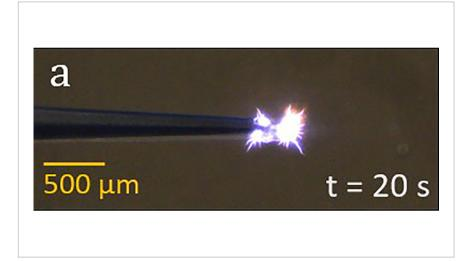
Fig. (a): Image of plasma discharge
