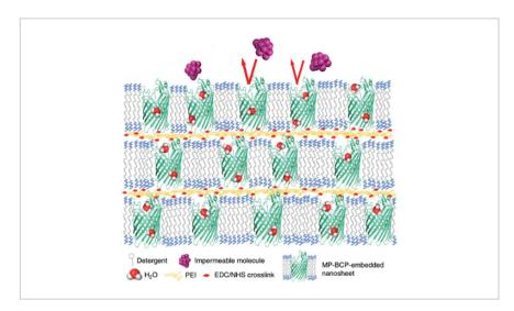
Schematic of layer-by-layer membrane fabrication procedure
