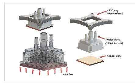
Hybrid microjet liquid-cooled heat sink
