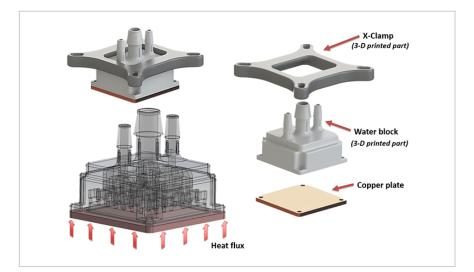
Hybrid microjet liquid-cooled heat sink
