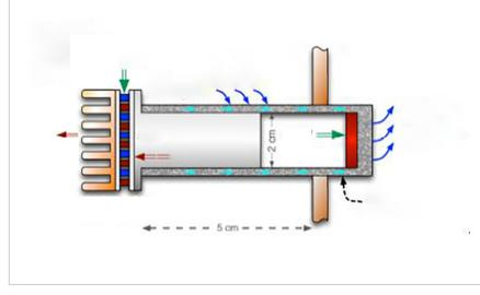
Schematic of solid-state dehumidifier
