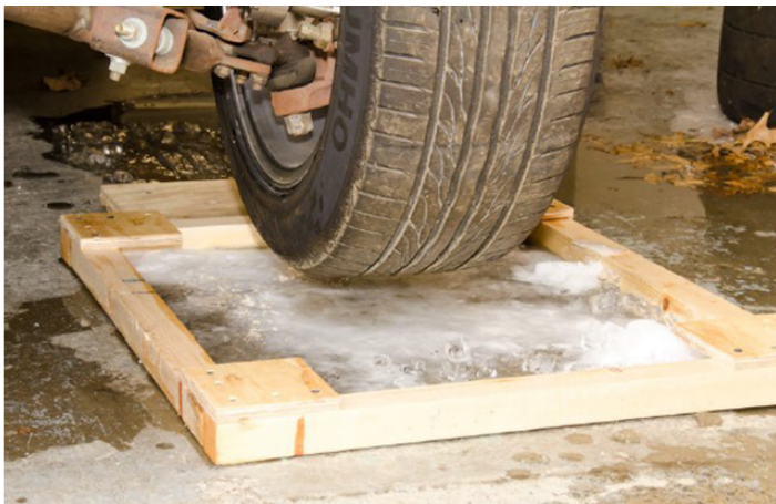
Experimental setup for scrub torque test
