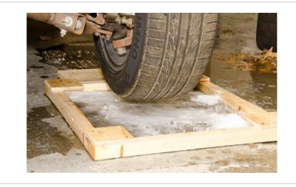
Experimental setup for scrub torque test
