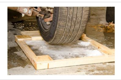
Experimental setup for scrub torque test
