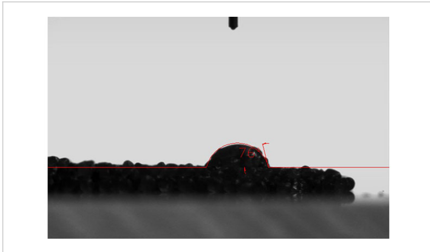
Water droplet on GNP proppant film
